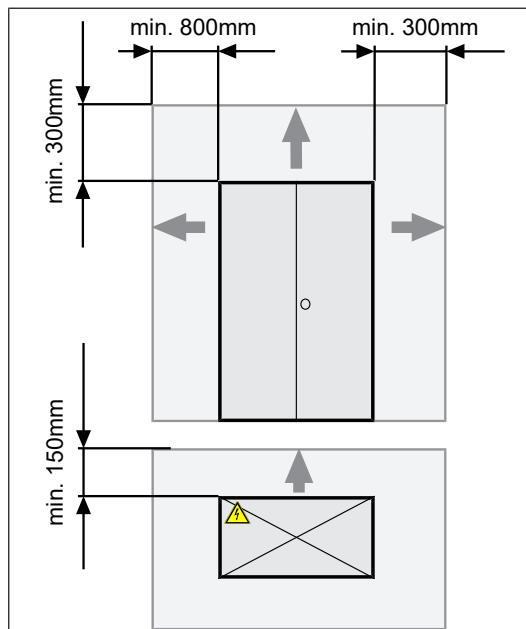
The installation site must be sufficiently level. Ensure that the system stands firmly in a 100 % vertical position and does not wobble.
