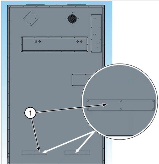
Depending on the air quality, dust can accumulate inside the base of the pressure chamber over time.
