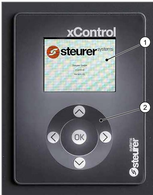
The following start-up screen appears once the device has been switched on. After a few seconds, this switches to the main screen and you can make your custom settings on the device.
