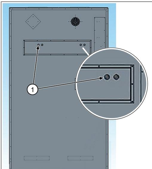
There are 2 excess temperature thermostats (Klixons) on the rear of the device. These are to protect the device and environment and may trip in certain circumstances.
